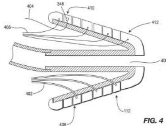
Figure 4 depicts a section of first end 112 of conductor portion 104. *Id.* ¶¶ 22, 33. Fiber optic cables 402 terminate in optically transparent elastomer 408 of first end 112 to allow the communication of light between fiber optic cable 402 and the tissue of the auditory canal wall. *Id.* ¶ 33.
