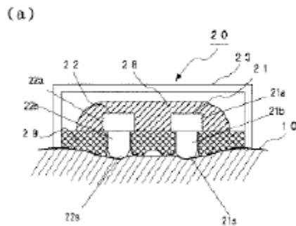
Figure 1(a) depicts pulse wave sensor 20 including light emitting device 21 and light receiving device 22, which are enclosed and supported by sensor case 23 and shell supporting member 29. *Id.* ¶ 9. Sensor 20 also includes light guide 21b extending from light emitting device 21 to direct infrared light to wrist 10 and light guide 22b extending to light receiving device 22 to
